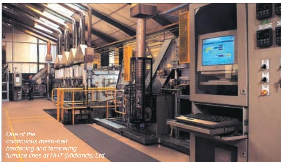
One of the continuous mesh-belt hardening and tempering furnace lines at HHT (Midlands) Ltd.
