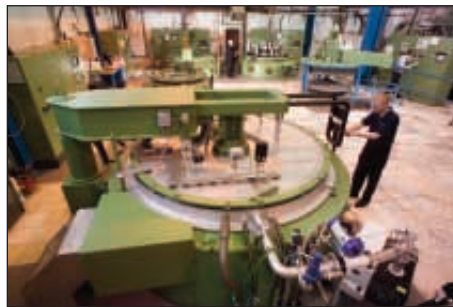
The new gas nitriding furnace at Bodycote Heat Treatments' Stockport site.
