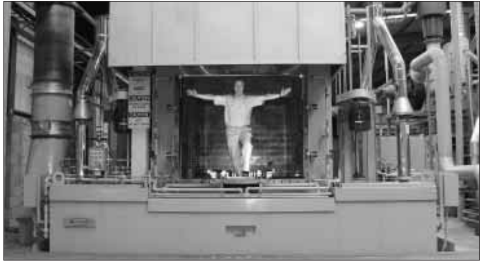
Managing Director Simon Day sizes up the new sealed-quench austempering installation at ADI Treatments.
