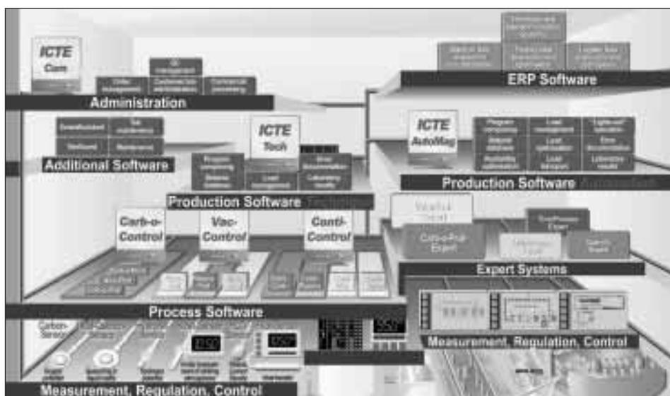
includes the programs that actually control, monitor and optimise furnace operation as well as record furnace data. These programs include *Carb-o-Control*, *Vac-Control* and *Conti-Control*.
