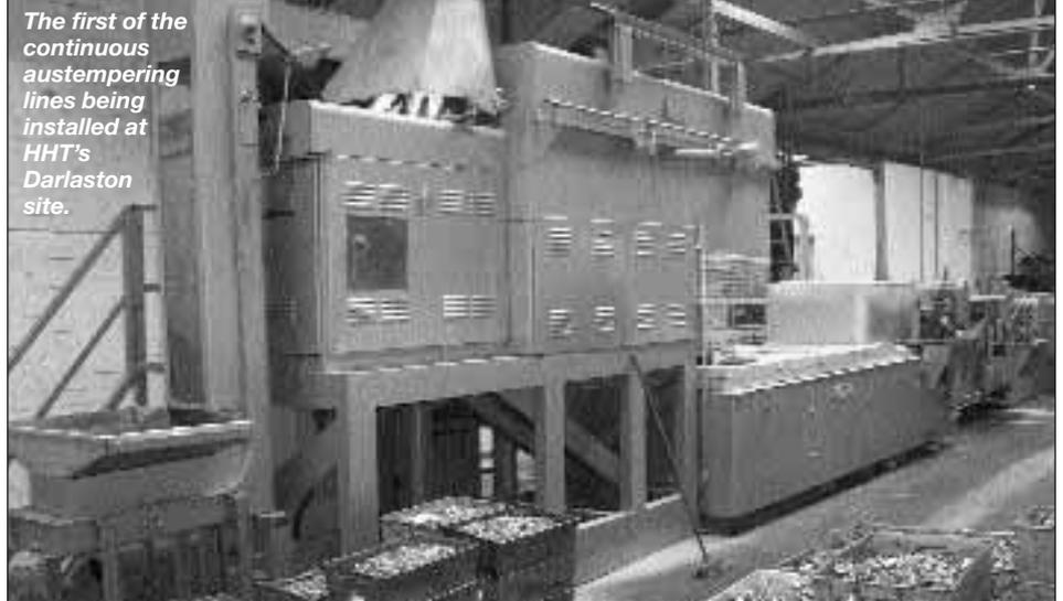
*The first of the continuous austempering lines being installed at HHT's Darlaston site.*
