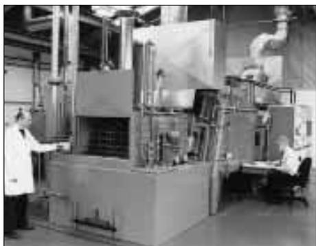
Reflecting the continuing success of TTI's Birmingham-based Nitrotec Services division, this Nitrotec cell was commissioned at the Group's Letchworth site last year. It provides additional capacity for the fast-expanding application of this range of advanced nitrocarburising processes, whilst meeting the need for wider geographical coverage.
